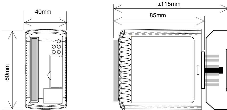
External dimensions of a typical module.
