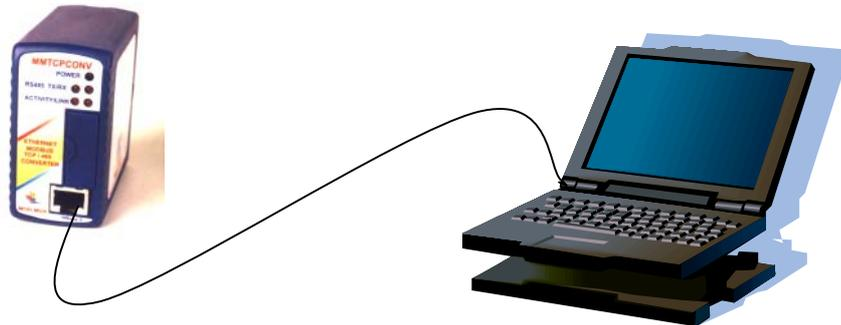
To setup your PC to connect directly to the MOD-MUX TCP Module, an IP address in the same range as the MOD-MUX TCP Module must be assigned to the PC. In Windows environments, this should be done as follows:
